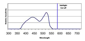
Use an appropriate safelight with a cut-off of no lower than 580nm – either a dark brown or red type.
