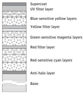
Total layer thickness (without base): 16 μm
