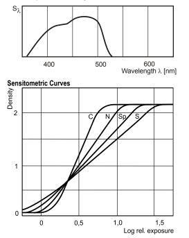
The above shown curves are valid for the glossy surface. Any other surface, namely the matt one, causes a decrease in the maximum density value. According to the ISO standard, the following sensitometric values correspond to the individual contrast grades:
